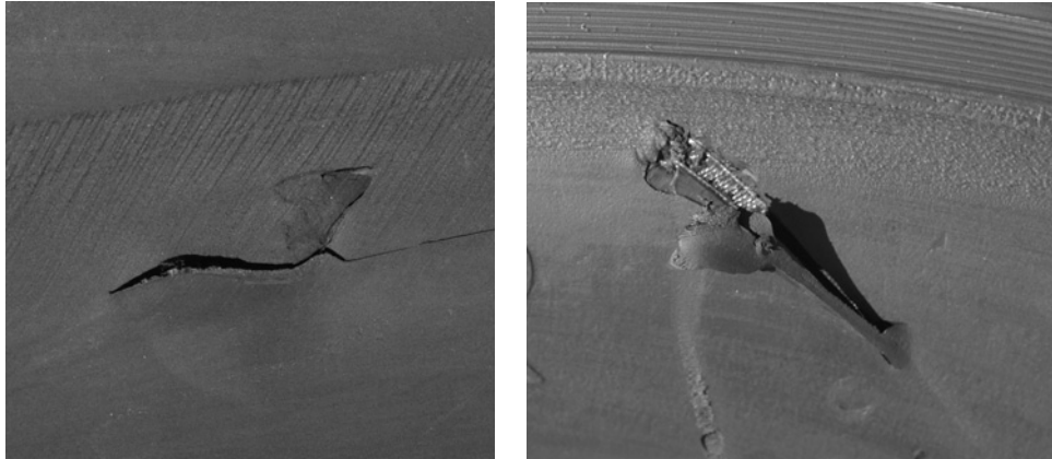
Figure 535. Sidewall FOD – Remove From Service (exposed cords)
