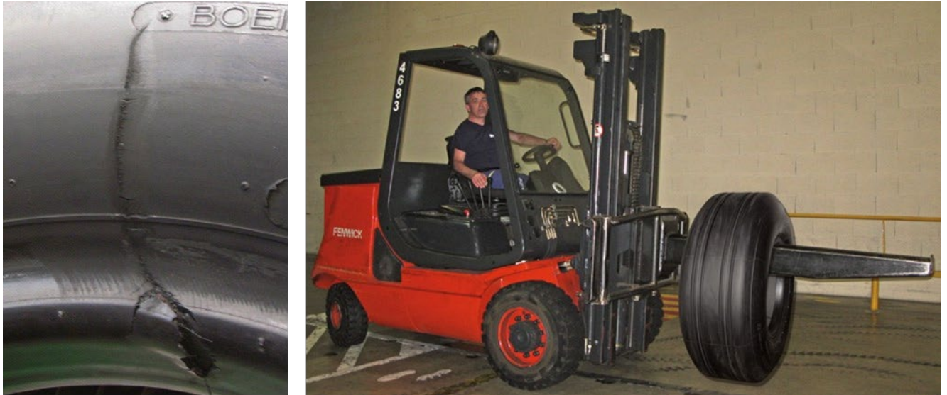
Figure 301. Damage From Lift Truck Forks (Left), Tires Can Be Lifted Through the Center (Right)
