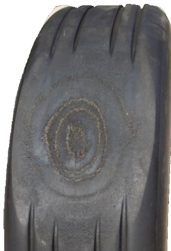
Exposed Reinforcing Plies
