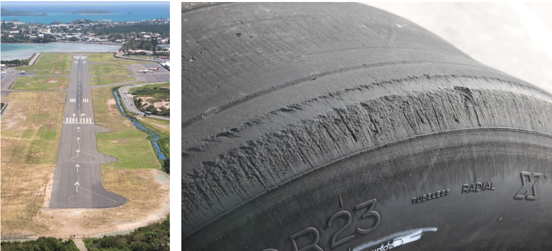
Figure 543. Lateral shoulder scratches from pivot turns
