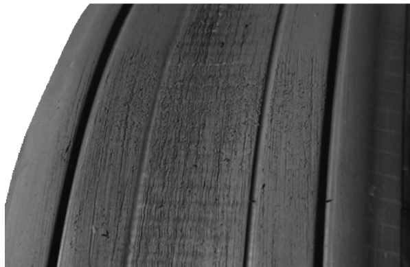
Figure 524. Aggressive Wear from Heavy Braking
