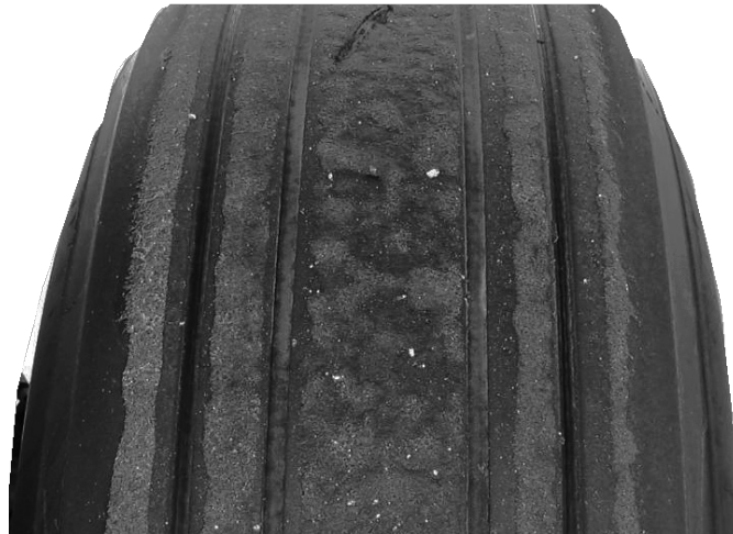
Figure 547. Contamination From Hydrocarbons
