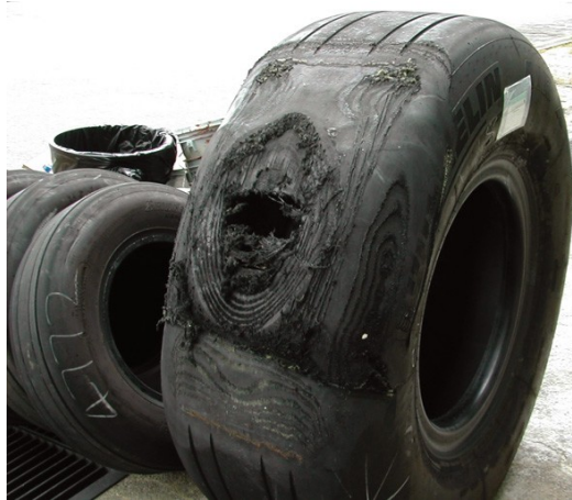
Figure 521. Flat Spot Resulting in Tire Rupture - Radial
