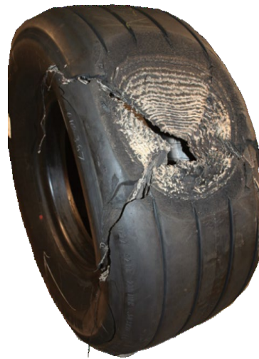
Flat Spot Causing Rupture
