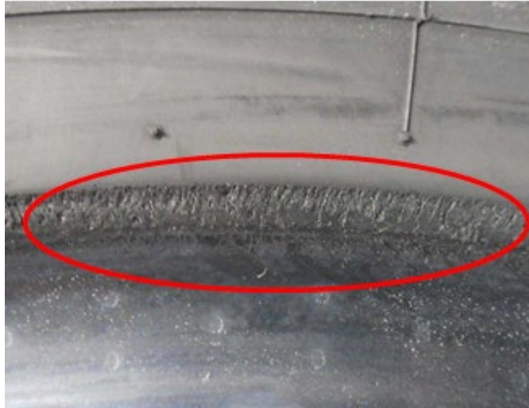
Figure 702. Retread Lower Sidewall Area Example
