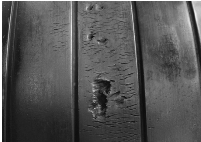
Figure 523. Chevron Cutting - Exposed Ply
